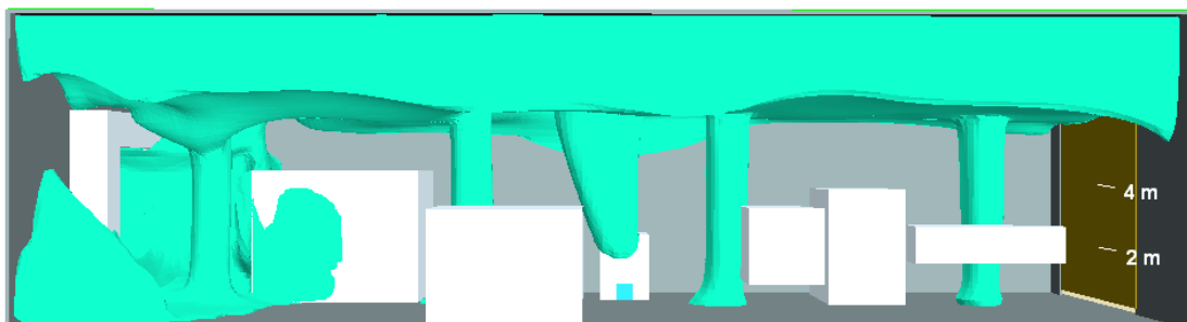
Figure 12 Zone with temperatures above 20°C (with four fans)
