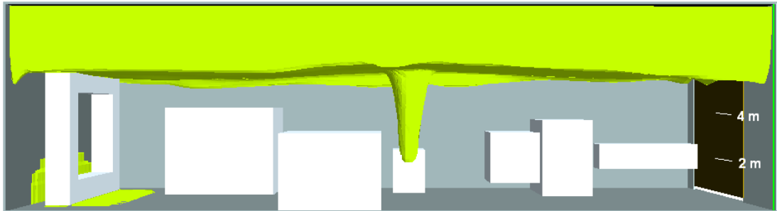
Figure 13 Zone with temperatures above 21°C (no fans)
