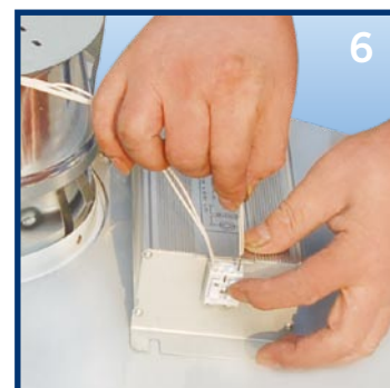
6 Connect the lamp wires to the ballast 将土星灯引出线与镇流器的输 出端连接
